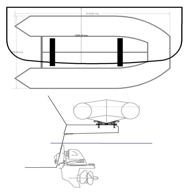
Mark holes for the 4 brackets, drill a 26mm hole for each braket, fasten bracket with 3 pcs 4,2x25mm screws.
